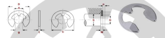
The most common form of radially fitted circlips for shafts with grooves. Provide a large shoulder on a relatively small shaft diameter. This range can be supplied stacked on rods for use with applicators and dispensers for rapid installation, thus resulting in sharply reduced assembly costs. Only the groove size is critical with this type of circlip, the shaft diameter can be varied widely.
